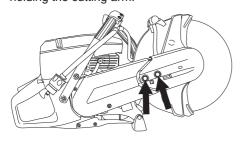
Screw the adjuster screw so that the square headed nut comes opposite the marking on the cover. This automatically ensures that the belt has the correct tension.
