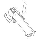
See instructions under the heading Start. Start the hedge trimmer and apply full throttle. Release the throttle trigger and check that the blades stop and remain stationary. If the blades move when the throttle trigger is in the idle position then the carburettor idle setting must be adjusted. See instructions under the heading Maintenance.
