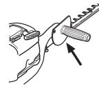
Check that the hand guard is fitted correctly.
