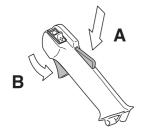
Make sure the throttle control is locked at the idle setting when the throttle lockout is released.
