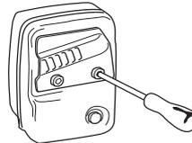
If the muffler on your machine is fitted with a spark arrestor mesh this must be cleaned regularly. A blocked mesh will cause the engine to overheat and may lead to serious damage.
