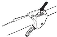
Start the engine and make sure the engine stops when you move the stop switch to the stop setting.
