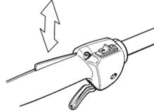
Check that the throttle control and throttle lockout move freely and that the return springs work properly.
