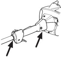
The machine's vibration damping system reduces the transfer of vibration between the engine unit/cutting equipment and the machine's handle unit.
