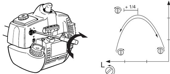
**CAUTION!** If the blades move while the engine is idling the T screw should be turned anti-clockwise until they stop.
