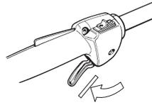
Press the throttle lockout and make sure it returns to its original position when you release it.
