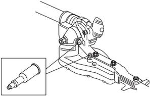
**CAUTION!** The gear housing must not be filled completely with grease. The grease expands as the machine heats up during operation. If the gear housing was completely filled with grease it could damage the seals and lead to leakage of grease.
