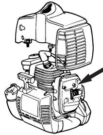
Some mufflers are equipped with a special spark arrestor mesh. If your machine has this type of muffler, you should clean the mesh at least once a week. This is best done with a wire brush.
