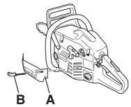
These reduce the flow of cooling air and prevent large amounts of snow from being sucked into the carburettor space.
