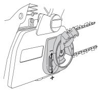
• Tighten the bar clutch by turning the knob clockwise.
