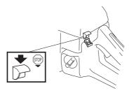
The engine is stopped by pushing the stop switch to the stop position.
