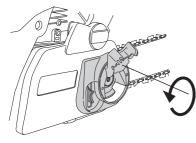
Adjust the tension on the chain by turning the wheel down (+) for tighter tension and up (-) to loosen the tension.
