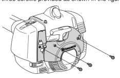
Remove the air filter and air filter cover from the machine. Fit the air filter and air filter cover supplied with the winter kit.
