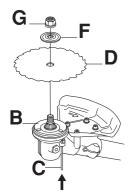
Fit the nut (G). The nut must be tightened to a torque of 35-50 Nm (3.5-5 kpm). Use the socket spanner in the tool kit. Hold the shaft of the spanner as close to the blade guard as possible. To tighten the nut, turn the spanner in the opposite direction to the direction of rotation (Caution! left-hand thread).
