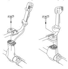
Put on the harness and hang the machine from the support hook. Now make a final adjustment so that the machine is in a comfortable working position when it hangs from the harness.
