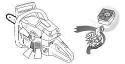
IMPORTANT! In order to maintain operation of the centrifugal cleaning system it must be regularly maintained. Clean the air intake to the starter, the fins on the flywheel, the space around the flywheel, inlet pipe and carburettor compartment.
