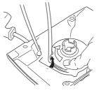
Undo the screw in the centre of the pulley and remove the pulley. Insert and fasten a new starter cord to the pulley.
