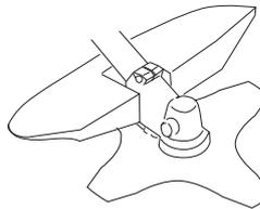
Check that the guard is undamaged and not cracked. Replace the guard if it has been exposed to impact or is cracked.
