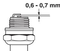
**CAUTION!** Always use the recommended spark plug type! Use of the wrong spark plug can damage the piston/cylinder. Check that the spark plug is fitted with a suppressor.
