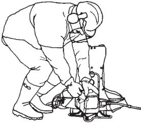
**CAUTION!** Do not put any part of your body in marked area. Contact can result in burns to the skin, or electrical shock if the spark plug cap has been damaged. Always use gloves. Do not use a machine with damaged spark plug cap.
