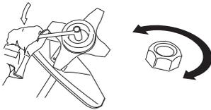
The nylon lining inside the locking nut must not be so worn that you can turn it by hand. The lining should offer a resistance of at least 1.5 Nm. The nut should be replaced after it has been put on approx. 10 times.
