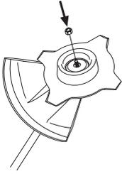
When fitting, tighten the nut in the opposite direction to the direction of rotation of the cutting attachment. To remove it, undo the nut in the same direction as the cutting attachment rotates. (CAUTION! The nut has a left-hand thread.) Tighten the nut using the socket spanner.
