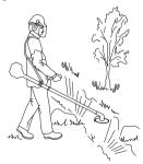
5 Take great care when cutting a tree that is in tension. A tree that is in tension may spring back to its normal position before or after being cut. If you position yourself incorrectly or make the cut in the wrong place the tree may hit you or the machine and cause you to lose control. Both situations can cause serious personal injury.
