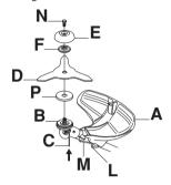
Screw the support cup (E) onto the output shaft threads (CAUTION! Left-hand thread). Tighten to a torque of 35-50 Nm (3.5-5.0 kpm). Use the socket spanner in the tool kit. Note that the locking pin (C) must remain inside the gear housing to lock the drive disk. Hold the shaft of the socket spanner as close to the blade guard/combination guard as possible.
