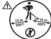
Machines fitted with saw blades or grass blades can be thrown violently to the side when the blade comes into contact with a fixed object. This is called blade thrust. The blade is capable of amputating an arm or leg. Always keep people and animals at least 15 metres from the machine.
