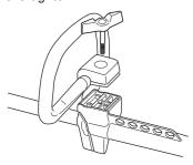
Put on the shoulder strap and hang the trimmer from the support hook. Now make a final adjustment so that the trimmer is in a comfortable working position when it hangs from the shoulder strap. Tighten the knob.
