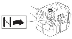
**Primer bulb:** Press the air purge repeatedly until fuel begins to fill the bulb. The bulb need not be completely filled.
