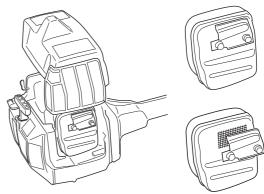
Some mufflers are equipped with a special spark arrestor screen. If your machine has this type of muffler, you should clean the screen at least once a week. This is best done with a wire brush.
