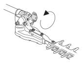
Press the cutting unit against the hedge or some other firm surface until the required angle is set.
