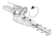
Adjust the angle with the help of the handle on the cutting unit.
