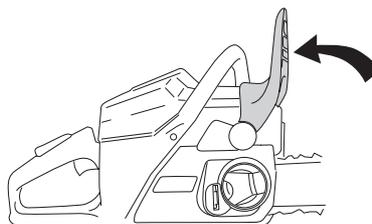
Remove the knob and remove the clutch cover (chain brake). Take off the transportation ring.
