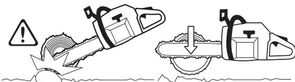
If it is possible (can you turn the log?) stop cutting about 2/3 of the way through the log.
