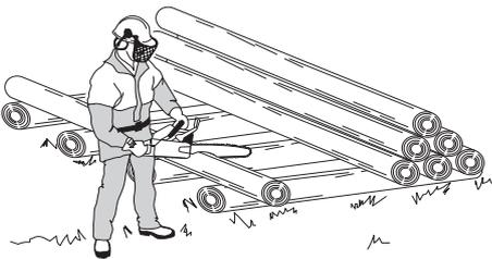
**The log is lying on the ground.** There is little risk of the chain jamming or the object splitting. However there is a risk that the chain will touch the ground when you finish the cut.
