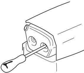
Some mufflers are equipped with a special spark arrester screen. If your machine has this type of muffler, you should clean the screen at least once a week. This is best done with a wire brush. A blocked screen will cause the engine to overheat and may lead to serious damage.
