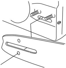
Tension the chain by turning the wheel down (+). The chain should be tensioned until it does not sag from the underside of the bar. See instructions under the heading Tensioning the chain.
