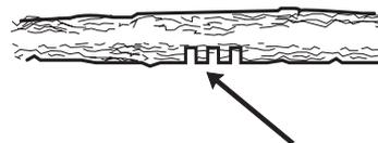
Continue to cut deeper until tree/limb bends and tension is released.
