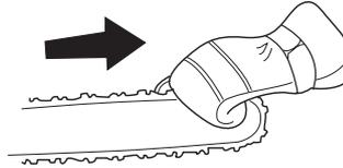
Note: If clutch cover is difficult to remove, replace bar nuts, engage brake and rerelease (an audible click will be heard if released properly).
