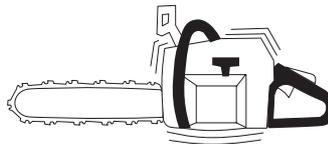
Make sure the vibration damping units are securely attached to the engine unit and handle unit.
