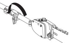
Push and hold the button (C). While securely holding the engine end, pull the attachment straight out of the coupling.
