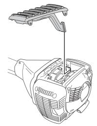
IMPORTANT! If the temperature rises above -5°C (23°F) or 0°C (32°F) respectively the machine MUST be restored to its normal set-up. Otherwise there is a risk of overheating, which can cause severe engine damage.
