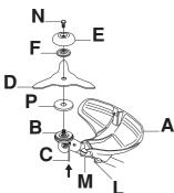
Screw the support cup (E) onto the output shaft threads (CAUTION! Left-hand thread). Tighten to a torque of 35-50 Nm (3.5-5.0 kpm). Use the socket spanner in the tool kit. Note that the locking pin (C) must remain inside the
