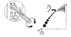
**CAUTION!** For optimum adjustment of the carburettor, contact a qualified dealer/service workshop that has a revolution counter at their disposal.
