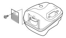
The muffler is designed to reduce the noise level and to direct the exhaust gases away from the operator. The exhaust gases are hot and can contain sparks, which may cause fire if directed against dry and combustible material.
