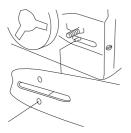
Tension the chain by turning the chain tensioning screw clockwise using the combination spanner. See instructions under the heading Tensioning the chain.
