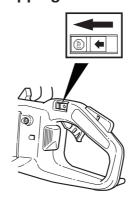
The engine is stopped by pushing the stop switch to the stop position.
