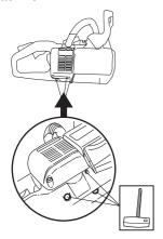
Some mufflers are equipped with a special spark arrestor screen. If your machine has this type of muffler, you should clean the screen at least once a week. This is best done with a wire brush. A blocked screen will cause the engine to overheat and may lead to serious damage.
