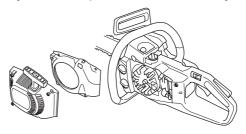
Clean the cooling system with a brush once a week, more often in demanding conditions. A dirty or blocked cooling system results in the machine overheating which causes damage to the piston and cylinder.
