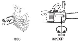
The chain is correctly tensioned when it does not sag from the underside of the bar, but can still be turned easily by hand. Hold up the bar tip and tighten the bar nuts with the combination spanner.
