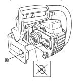
Fit the bar over the bar bolts. Place the bar in its rearmost position. Place the chain over the drive sprocket locate it in the groove on the bar. Begin on the top edge of the bar.
