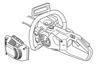
Pull out the cord approx. 30 cm (12 inches) and hook it into the notch in the rim of the pulley. Release the recoil spring by letting the pulley rotate slowly backwards.
