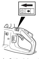
Choke: Set the choke control in the choke position.
