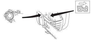
Make sure that the edges of the cutting links are facing forward on the top edge of the bar.
