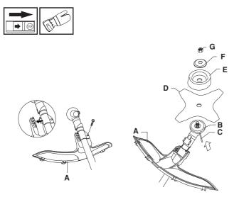
Hook the blade guard/combination guard (A) onto the fitting on the shaft and secure with the bolt. CAUTION! Ensure that the guard extension is removed.
