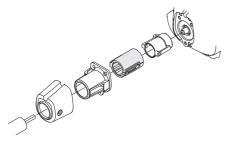
Regularly check the vibration damping units for cracks or deformation.
