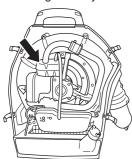
The muffler is equipped with a special spark arrestor screen. The spark arrestor screen should be cleaned once a month. This is best done with a wire brush.
