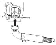
Also pay attention to the stops located on the pipe bend and the fan's outlet pipe. Ensure that the stop on the pipe bend comes in front of the stop on the outlet pipe.
