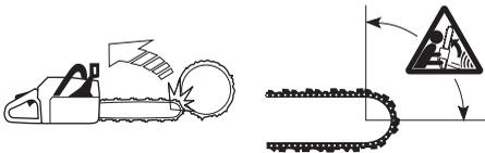
Kickback always occurs in the cutting plane of the bar. Normally the chain saw and bar are thrown backwards and upwards towards the user. However, the chain saw may move in a different direction depending on the way it was being used when the kickback zone of the bar touched the object.
