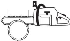
There are methods for felling trees with a diameter larger than the bar length. However these methods involve a much greater risk that the kickback zone of the bar will come into contact with the tree.
