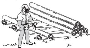
**The log is lying on the ground.** There is little risk of the chain jamming or the object splitting. However there is a risk that the chain will touch the ground when you finish the cut.
