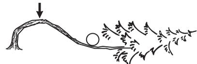
Decide which is the safest way to release the tension and whether you are able to do it safely. In complicated situations the only safe method is to put aside your chain saw and use a winch.
