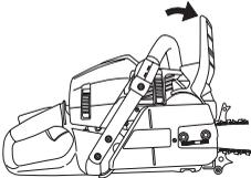
**Ignition; choke:** Set the choke control in the choke position. This should automatically set the stop switch to the start position.
