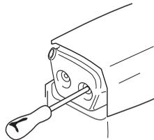
Some mufflers are equipped with a special spark arrestor screen. If your machine has this type of muffler, you should clean the screen at least once a week. This is best done with a wire brush. A blocked screen will cause the engine to overheat and may lead to serious damage.
