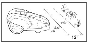
If the working area borders against a flat path or the like that lies level with the lawn, it is possible to allow Automower to run a little over the path. The boundary wire should then be laid 4" from the edge of the path.
