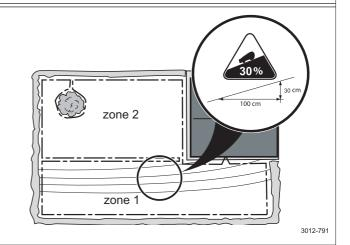
Two gardens with the area 0,04 acre. Two separate installations each with a loop generator/charger have been made, where the mower may be moved between gardens.
