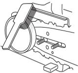
Regularly check that the brake band is at least 0.6 mm thick at its thinnest point.
