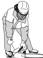
Push in the starter cord as soon as the engine fires and keep pulling until the engine starts. When the engine starts, quickly apply full throttle; the throttle start lock will automatically disengage.
