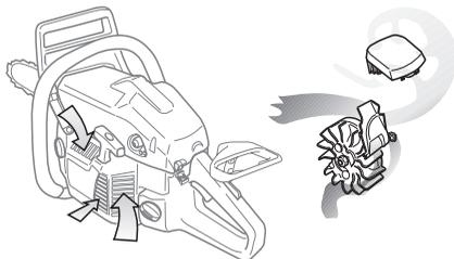
**IMPORTANT!** In order to maintain operation of the centrifugal cleaning system it must be regularly maintained. Clean the air intake to the starter, the fins on the flywheel, the space around the flywheel, inlet pipe and carburettor compartment.
