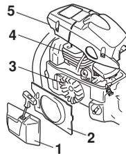
Clean the cooling system with a brush once a week, more often in demanding conditions. A dirty or blocked cooling system results in the machine overheating which causes damage to the piston and cylinder.
