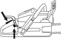
Note! Reactivate the chain brake by pushing the front hand guard back towards the front handle. The chain saw is now ready for use.
