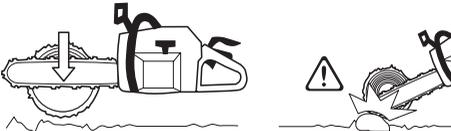
If it is possible (can you turn the log?) stop cutting about 2/3 of the way through the log.
