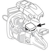
The filter can be cleaned more thoroughly by washing it in water and detergent.
