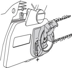
The chain is correctly tensioned when it does not sag from the underside of the bar, but can still be turned easily by hand. Hold up the bar tip and tighten the bar knob by turning the knob clockwise.
