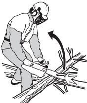
Have control over the workpiece. If the pieces you intend to cut are small and light, they can jam in the saw chain
