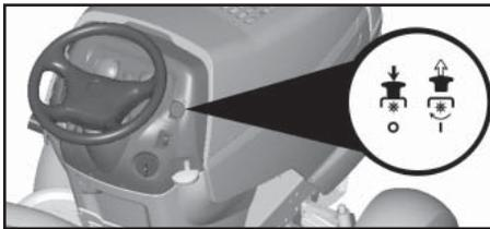
(↓) ATTACHMENT CLUTCH SWITCH PULL OUT TO "ENGAGE"
