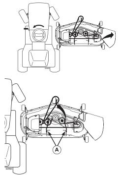
**NOTE:** Be sure mower side suspension arms (A) are pointing forward before sliding mower under tractor.
