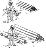
The log is lying on the ground. There is little risk of the chain jamming or the object splitting. However there is a risk that the chain will touch the ground when you finish the cut.
