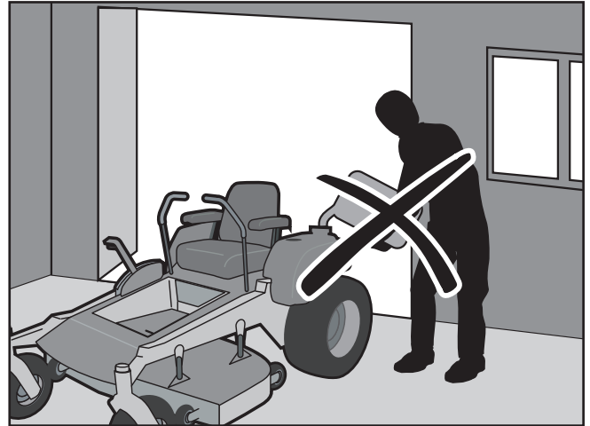
Never fill the fuel tank indoors
