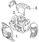
The cooling system consists of:
