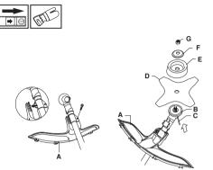
Hook the blade guard/combination guard (A) onto the fitting on the shaft and secure with the bolt.
