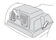
Lubricate the joints and bearings on the left side with an oilcan.
