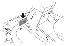
2 Carefully press down one of the pedals until the required speed is obtained. Pedal (1) is used to drive forwards, and pedal (2) to drive backwards.
