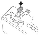
4 If the engine is cold move the choke lever backwards to its end position.
