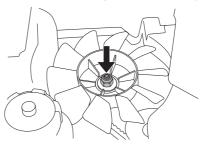
7 Remove the belt from the hydrostatic transmission pulley.
