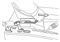
4 Select the required cutting height (1-7) with the cutting height lever.
