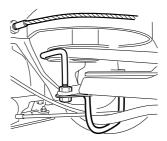
5 Pull off the centre belt from the engine's pulley and pull out the rear section.
