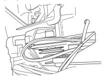
6 Fit the hose holder in the middle and the belt guide for the centre belt.
