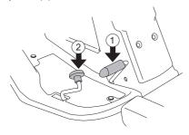
3 Press in the lock button on the mechanical lifting lever and lower the cutting unit.
