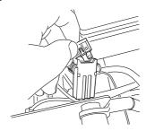
The fuse for the power outlet is placed under the ignition switch, behind the side plate on the control panel. Type: Flat pin, 7,5 A.
