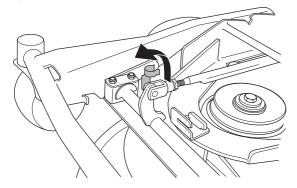
Remove the bolt so the track rod is released in one end.
