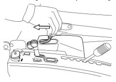
The unit can then be secured in the raised position if necessary by moving the mechanical lifting lever backwards to the lock position.
