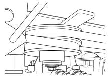
4 Reset the cutting unit from service position to mowing position.
