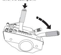
If the cutting unit does not lower completely, or if the blades do not rotate, lower the cutting unit completely using the hydraulic lifting lever. In order to ensure that the hydraulic cylinder is in the outer position, hold the lever in the forward position for a half to one second.
