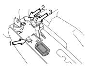
The lights are switched on and off using the power switch (1) on the control panel.
