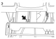
4 Push the deck in and put the front guide plugs in the grooves on the equipment frame, one on each side.
