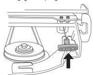
Loosen on the cutting height stay and place in the holder.
