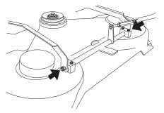
6 Remove the screws on the cutting cover. Lift the unit frame and remove the cutting unit cover.
