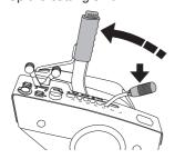
3 Remove the front hood by removing the pin. (There are complete instructions on using the service position inside the front hood).
