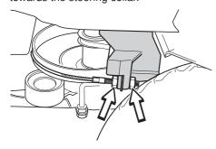
Hold the cable, for example using an adjustable wrench, so that it does not twist.
