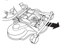
7 Lift the unit until it stops and a clicking sound is heard. The unit locks automatically in the vertical position.
