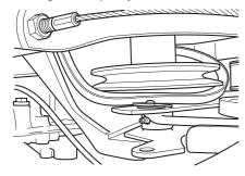
8 Pull out the belt through the opening under the pivot bearing and past the belt tensioner's disc.
