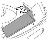
Work the pedals and lubricate the moving parts with an oilcan. Lubricate the cables for the brake and drive pedals using an oil can.
