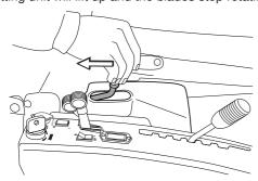
Secure the cutting unit if necessary using the mechanical lifting lever.
