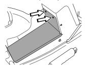
2 Check the tension of the steering wires by squeezing them together by the arrows as illustrated. It should be possible to push them together so that the distance between them is half as much, without using unnecessary force.
