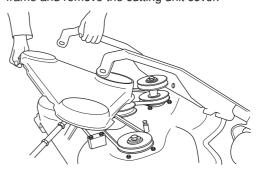
7 Loosen the spring that tensions the V-belt and pry off the belt
