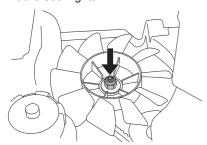
5 Check that the centre belt is fitted correctly on its front pulley and fit the centre belt on the engine's pulley.
