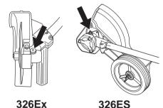
The grease in the bevel gear does not normally need to be changed except if repairs are carried out.
