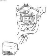
Some mufflers are equipped with a special spark arrestor screen. If your machine has this type of muffler, you should clean the screen at least once a week. This is best done with a wire brush.
