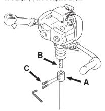
2 Fit the screws (C) and tighten using the Allen key provided.
