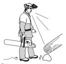
Take great care when cutting a tree that is in tension. A tree that is in tension may spring back to its normal position before or after being cut. If you position yourself incorrectly or make the cut in the wrong place the tree may hit you or the machine and cause you to lose control. Both situations can cause serious personal injury.
