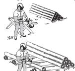
The log is lying on the ground. There is little risk of the chain jamming or the object splitting. However there is a risk that the chain will touch the ground when you finish the cut.
