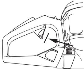
Press the throttle lockout and make sure it returns to its original position when you release it.
