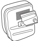
On mufflers without a catalytic converter the mesh should be cleaned weekly, or replaced if necessary. On mufflers fitted with a catalytic converter the mesh should be checked, and if necessary cleaned, monthly. **If the mesh is damaged it should be replaced.** If the mesh is frequently blocked, this can be a sign that the
