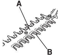
Check that the blade guard is not damaged or distorted. Replace the blade guard if it is bent or damaged.
