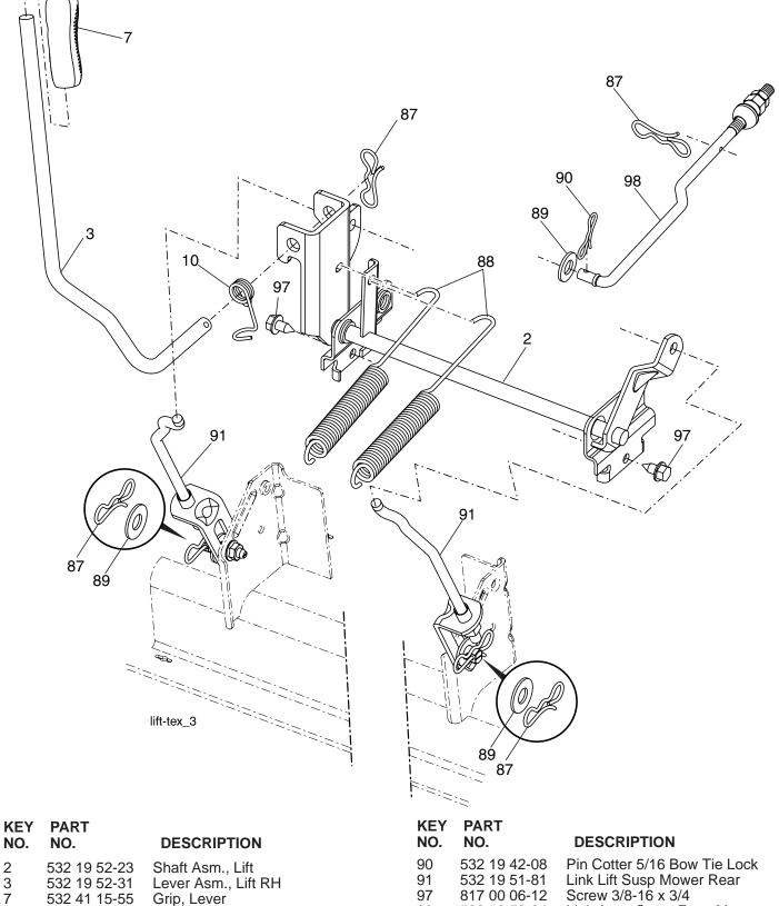
Screw 3/8-16 x 3/4 97 817 00 06-12 Link Asm. Susp. Front Mower 532 19 52-64 98
