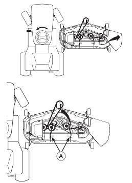
**NOTE:** Be sure mower side suspension arms (A) are pointing forward before sliding mower under tractor.
