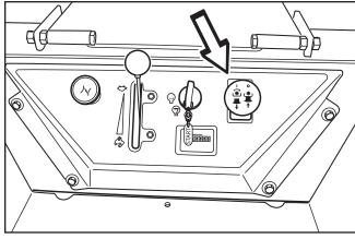
Disengaging the mower deck
