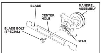
**IMPORTANT:** Special blade bolt is heat treated.
