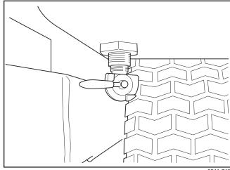
Fuel shut off valve in OFF position
