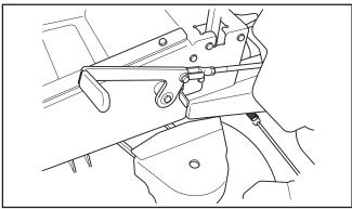
The parking brake in the disengaged position
