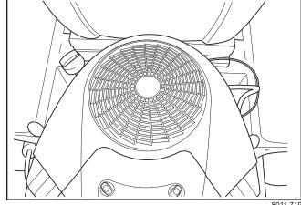
Check and clean the cooling air intake
