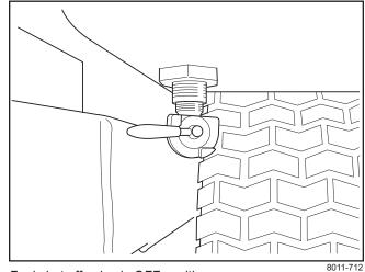
Fuel shut off valve in OFF position
