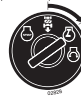
Engine "ON" Position (Normal Operating)
