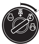
Engine "ON" Position (Normal Operating)
