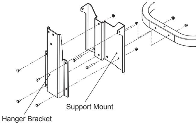
hanger assembly. Set reinforcement plates to the outside of the tank brackets and fasten front end of support strap to tank bracket and reinforcement plate with round head bolt. Secure front end of reinforcement plate to tank bracket with hex bolt. Fully secure all mounting hardware. See illustration.
