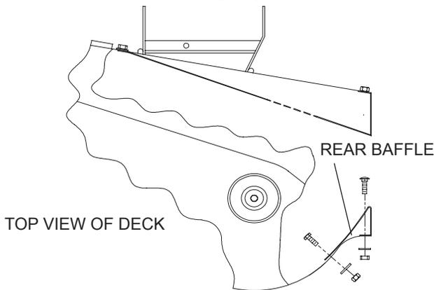
of discharge chute. From inside deck, install  $\frac{1}{4}$ -20 x  $\frac{3}{4}$ " bolt through slotted hole in baffle and extend through deck wall. Attach  $\frac{1}{4}$  washer and  $\frac{1}{4}$ -20 nyloc nut. Install  $\frac{5}{16}$ -18 x  $\frac{3}{4}$ " carriage bolt in square hole in the same manner and attach  $\frac{5}{16}$  washer and  $\frac{5}{16}$ -18 nyloc nut. Lift baffle to top of slot and tighten hardware.
