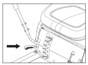
Mower deck's lifting lever
