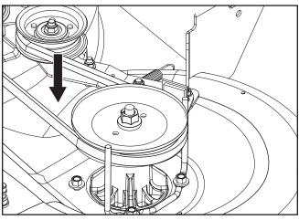
Check deck belt for excessive wear
