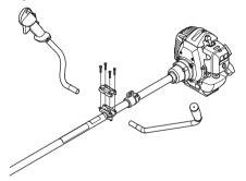
· Fit the protective sleeve as shown in the diagram.
