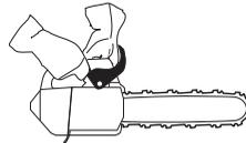
Apply full throttle and activate the chain brake by tilting your left wrist forward onto the front hand guard. Do not let go of the front handle. **The chain should stop immediately.**
