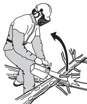
Have control over the workpiece. If the pieces you intend to cut are small and light, they can jam in the saw chain and be thrown towards you. Even if this does not need to be a danger, you may be surprised and lose control of the saw. Never saw stacked logs or branches without first separating them. Only saw one log or one piece at a time. Remove the cut pieces to keep your working area safe.
