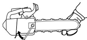
When fitting a new chain, the chain tension has to be checked frequently until the chain is run-in. Check the chain tension regularly. A correctly tensioned chain ensures good cutting performance and long life.
