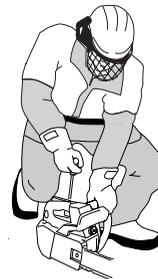
Push down the choke control as soon as the engine fires which can be heard through a "puff" sound. Keep on pulling the cord powerfully until the engine starts. When
