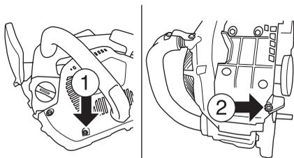
Push the muffler cover as shown in the picture.
