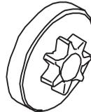
Regularly check the degree of wear on the drive sprocket. Replace if wear is excessive. Replace the drive sprocket whenever you replace the chain.
