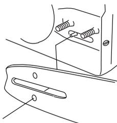
Tension the chain by turning the chain tensioning screw clockwise using the combination spanner. The chain should be tensioned until it does not sag from the underside of the bar, but can still be turned easily by hand. Hold up the bar tip and tighten the bar nuts with the combination spanner.
