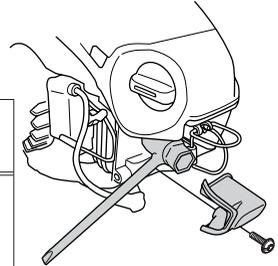
Note! Always use the recommended spark plug type! Use of the wrong spark plug can damage the piston/cylinder. Check that the spark plug is fitted with a suppressor.
