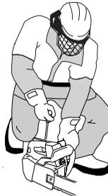
Push down the choke control as soon as the engine fires which can be heard through a "puff" sound. Keep on pulling the cord powerfully until the engine starts. When
