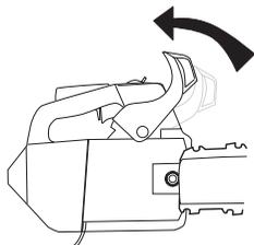
Unscrew the bar nut and remove the clutch cover (chain brake). Take off the transportation guard.
