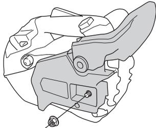
Fit the bar over the bar bolts. Place the bar in its rearmost position. Place the chain over the drive sprocket locate it in the groove on the bar. Begin on the top edge of the bar.
