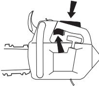
Note! Reactivate the chain brake by pushing the front hand guard back towards the front handle. The chain saw is now ready for use.
