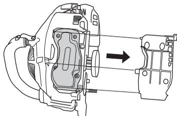
Loosen the screws and nuts. Remove and check that the muffler is ok.
