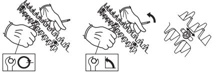
When the blades are correctly adjusted the play between the blades should be 0,2–0,4 mm, measured at the screws.
