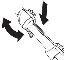
See instructions under the heading Start. Start the hedge trimmer and apply full throttle. Release the throttle trigger and check that the blades stop and remain stationary. If the blades move when the throttle trigger is in the idle
