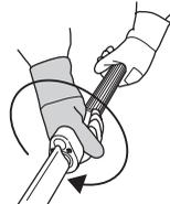
**CAUTION!** When the stop position has been passed the blades are blocked, do not try to cut with the cutting unit in this position.
