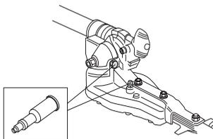
**CAUTION!** The gear housing must not be filled completely with grease. The grease expands as the machine heats up during operation. If the gear housing was completely filled with grease it could damage the seals and lead to leakage of grease.
