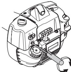
The blades must also remain stationary when the choke control is in the start throttle position.
