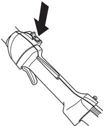
**CAUTION!** The stop switch automatically returns to the start position. In order to prevent unintentional starting, the spark plug cap must be removed from the spark plug when assembling, checking and/or performing maintenance.
