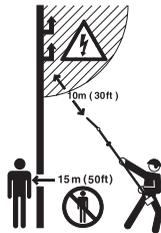
This machine can be dangerous! The operator of the machine must ensure, while working, that no persons or animals come closer than 15 metres.
