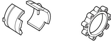
Regularly check the vibration damping units for cracks or deformation. Check that the vibration damping element is undamaged and securely attached.
