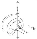
5 Now make a final adjustment to give yourself a comfortable working position. Tighten the screw. CAUTION! The loop handle and hand guard must not be fitted behind the arrow marked on the shaft.
