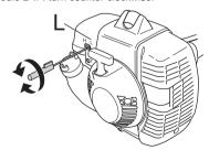
**CAUTION!** If the cutting attachment rotates when the engine is idling the idle adjustment screw T should be turned anti-clockwise until the cutting attachment stops.
