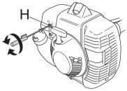
Note that the engine should be loaded when you adjust the high speed jet H. You should therefore fit the trimmer head T35 (2.7 mm cord) before adjusting the high speed jet. The cord length should be standard, i.e. to the knife on the trimmer guard.
