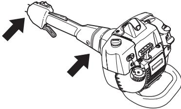
The machine's vibration damping system reduces the transfer of vibration between the engine unit/cutting equipment and the machine's handle unit.
