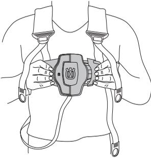
Check that the harness straps are correctly positioned. Once the harness and machine have been adjusted, check that the harness quick release works correctly.
