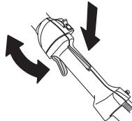
See instructions under the heading Start. Start the hedge trimmer and apply full throttle. Release the throttle trigger and check that the blades stop and remain stationary. If the blades move when the throttle trigger is in the idle position then the carburettor idle setting must be adjusted. See instructions under the heading Maintenance.
