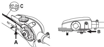
Tension the chain by turning the chain tensioning screw clockwise. Use a combination spanner or turn by hand.
