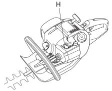
Apply full throttle and turn the high speed jet H very slowly clockwise until the engine slows down. Then turn the high speed jet H very slowly anticlockwise until the engine starts to run unevenly. Now turn the high speed jet H slowly clockwise a little way until the engine runs smoothly.
