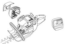
Some mufflers are equipped with a special spark arrestor screen. If your machine has this type of muffler, you should clean the screen at least once a week. This is best done with a wire brush.
