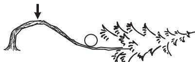
Decide which is the safest way to release the tension and whether you are able to do it safely. In complicated situations the only safe method is to put aside your chain saw and use a winch.
