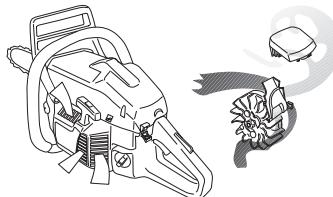
**IMPORTANT!** In order to maintain operation of the centrifugal cleaning system it must be regularly maintained. Clean the air intake to the starter, the fins on the flywheel, the space around the flywheel, inlet pipe and carburetor compartment.
