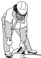
If the machine is fitted with a decompression valve (A): Press the valve to reduce the pressure in the cylinder and make starting easier. You should always use the decompression valve when starting the machine. Once
