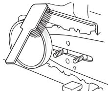
Regularly check that the brake band is at least 0.024 inch (0.6 mm) thick at its thinnest point.
