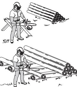
**The log is lying on the ground.** There is little risk of the chain jamming or the object splitting. However there is a risk that the chain will touch the ground when you finish the cut.
