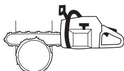
There are methods for felling trees with a diameter larger than the bar length. However these methods involve a much greater risk that the kickback zone of the bar will come into contact with the tree.
