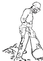
Keep the trunk between you and the chain saw as you move along the trunk.
