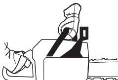
Apply full throttle and activate the chain brake by tilting your left wrist forward onto the front hand guard. Do not let go of the front handle. **The chain should stop immediately.**
