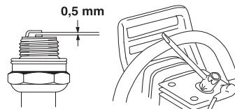
Note! Always use the recommended spark plug type! Use of the wrong spark plug can damage the piston/cylinder. Check that the spark plug is fitted with a suppressor.
