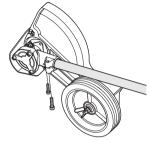
Tighten the two screws.
