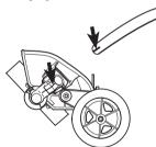
Position the angle gear so that its slot is aligned with the line on the supporting tube.
