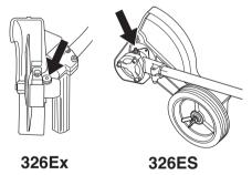
The grease in the bevel gear does not normally need to be changed except if repairs are carried out.
