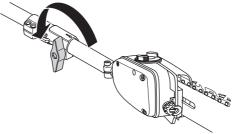
Push and hold the button (C). While securely holding the engine end, pull the attachment straight out of the coupling.
