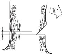
Set the spike bumper (if one is fitted) just behind the felling hinge. Use full throttle and advance the chain/bar slowly into the tree. Make sure the tree does not start to move in the opposite direction to your intended felling direction. Drive a wedge or breaking bar into the cut as soon as it is deep enough.
