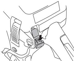
CAUTION! The start/stop switch automatically returns to run position. In order to prevent unintentional starting, the spark plug cap must be removed from the spark plug when assembling, checking and/or performing maintenance.
