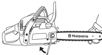
When fitting a new chain, the chain tension has to be checked frequently until the chain is run-in. Check the chain tension regularly. A correctly tensioned chain ensures good cutting performance and long life.
