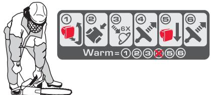
As the chain brake is still engaged the speed of the engine must be set to idling as soon as possible, this is achieved by disengaging the throttle lock. Disengagement is done by gently touching on the throttle trigger. This prevents unnecessary wear to the clutch, clutch drum and brake band. Allow the machine to idle a few seconds before giving full throttle.
