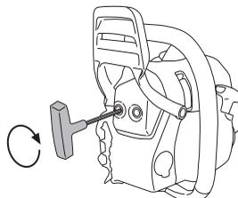
Some mufflers are equipped with a special spark arrestor mesh. If your machine has this type of muffler, you should clean the mesh at least once a week. This is best done with a wire brush. A blocked mesh will cause the engine to overheat and may lead to serious damage.
