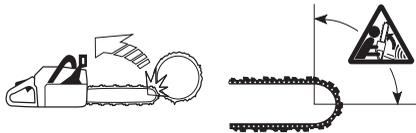
Cutting with the bottom edge of the bar, i.e. from the top of the object downwards, is known as cutting on the pull stroke. In this case the chain saw pulls itself towards the tree and the front edge of the chain saw body rests naturally on the trunk when cutting. Cutting on the pull stroke gives the operator better control over the chain saw and the position of the kickback zone.
