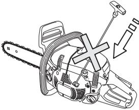
**Note!** Reactivate the chain brake by pushing the front hand guard back towards the front handle. The chain saw is now ready for use.
