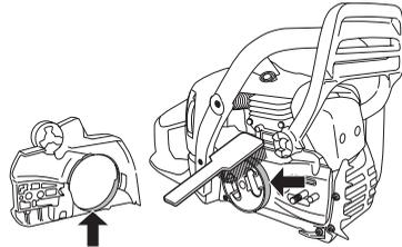
Regularly check that the brake band is at least 0.6 mm thick at its thinnest point.
