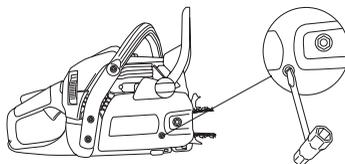
The chain is correctly tensioned when it does not sag from the underside of the bar, but can still be turned easily by hand. Hold up the bar tip and tighten the bar nuts with the combination spanner.
