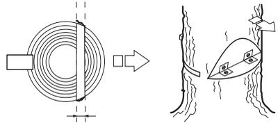
All control over the felling direction is lost if the felling hinge is too narrow or non-existent, or if the directional cuts and felling cut are badly placed.
