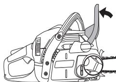
Loosen the chain tensioner wheel and remove the clutch cover (chain brake). Remove the transport guard.
