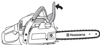
Remove the bar nuts and remove the clutch cover (chain brake). Take off the transportation ring (A).
