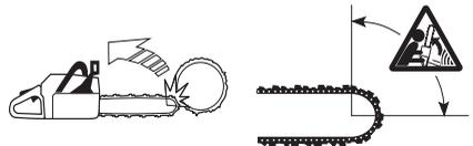
Kickback always occurs in the cutting plane of the bar. Normally the chain saw and bar are thrown backwards and upwards towards the user. However, the chain saw may move in a different direction depending on the way it
